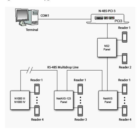
This configuration supports a combined total of 31 N1000 III, N1000 IV, NetAXS, NetAXS-123, and NS2 panels per Multidrop line.
